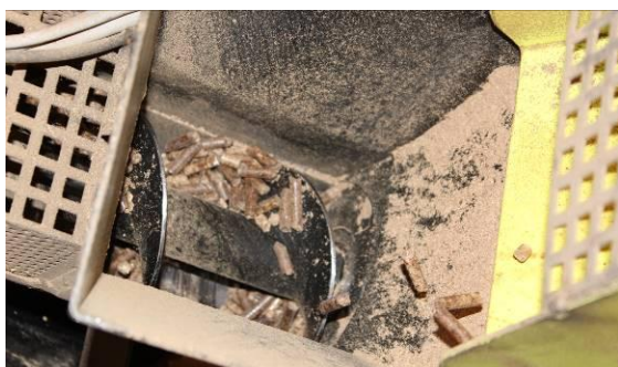
Figure 11: A further development of the micro plant can foresee a press for pellet production, fed with the previously produced wood chips.
