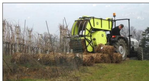
Figure 3: The bales' accumulator is able to unload automatically the 7 bales stored into the tunnel, while the bale contained into the baler chamber is discharged at the end of this operation, independently.
