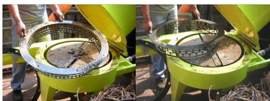
Figure 6: the grids used during the tests were 26 mm (left) and 45 mm (right) diameter, respectively.
