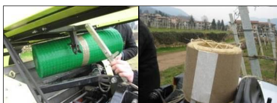
Figure 2: The baler was used, alternatively, with a net tying system (left) and a twine knotter (right) in order to obtain bales secured with different products.
