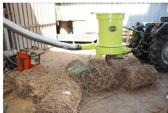
Figure 5: The shredder prototype used for the test was powered by the same tractor used during the field tests and connected to a silo by the conveyor 150 mm diameter supplied.
