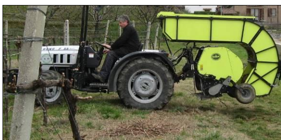
Figure 1: The harvest machinery combination composed of a narrow-track tractor, a small diameter round baler and a baler accumulator.
